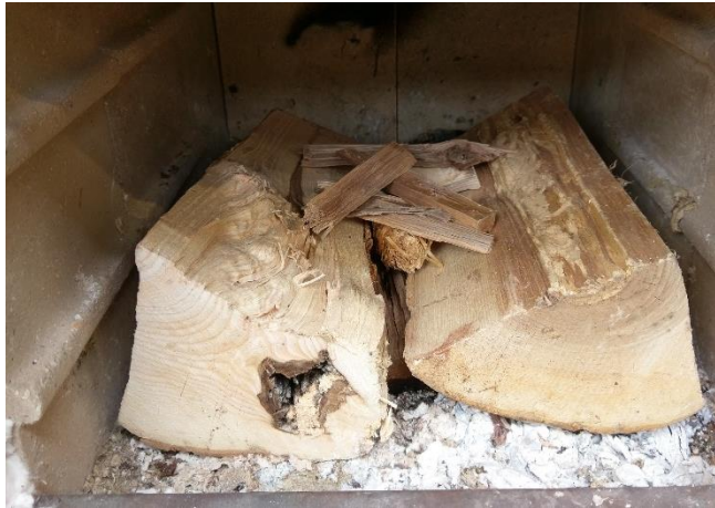
Figure 5 Fire Lighter and Kindling in Place
